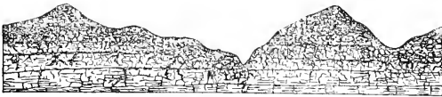
FIG. 17. Diagram showing the relation of mantle rock to the underlying rock from which it was derived. (Courtesy of U. S. Geol. Surv.)
